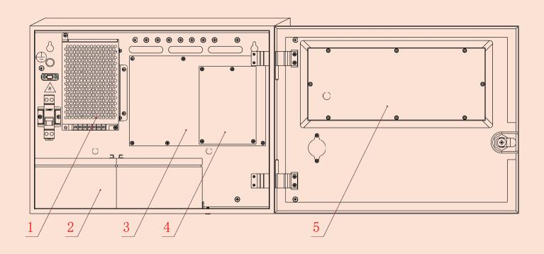
AC/DC power module ② Batteries ③ Main control board and power board
